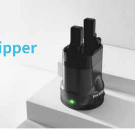
DH-Robotics PGC series of collaborative parallel electric grippers is an electric gripper mainly used in cooperative manipulators. It has the advantages of high protection level, plug and play, large load and so on. The PGC series combines precision force control and industrial aesthetics. In 2021, it won two industrial design awards, the Red Dot Award and the IF Award.
